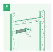
5. You can use cut strips to finish your toilet installation above and on the sides. Reinforce the corner joints and the joint between the wall and floor covering with self-adhesive fiberglass tape.
